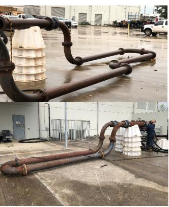
1.5D back-to-back bends: S and B2B20% restriction: full bore and plane bore
